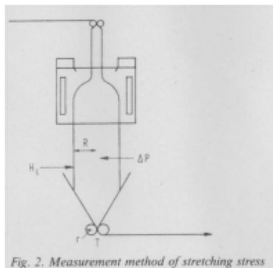
The force balance on the double bubble tubular film is developed from membrane theory. The membrane theory leads to a balance of forces on the film between positions Z and take-up position L. This has the form:
