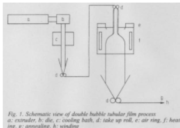
By using an extruder ( $L/D=25$ ) with the diameter of 115mm as well as a circular die with the diameter 300mm and lip clearance of 1 mm, non-stretched film for large scale production machine was produced at the condition of the resin temperature 265 °C, blow-up ratio of 1.1, and with a water-cooling ring having the diameter of 330mm.
